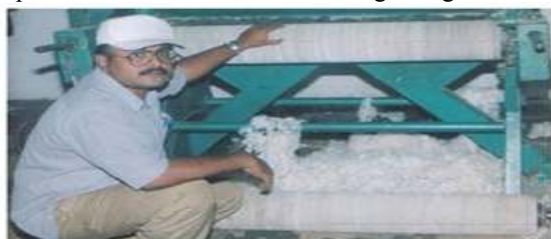
Figure-4: Seed-Cotton Ginning Using Green Design Rollers
